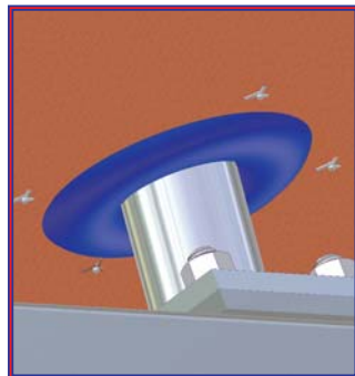
Underside of Roof Support Post Showing Hold-Down Ring Lock Rivets
