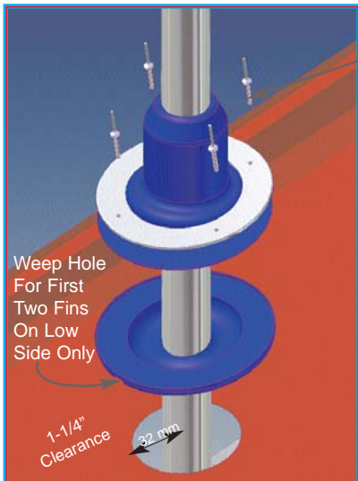
Exploded View Showing Thaler D-100 EPDM Flexible Flashing Assembly
